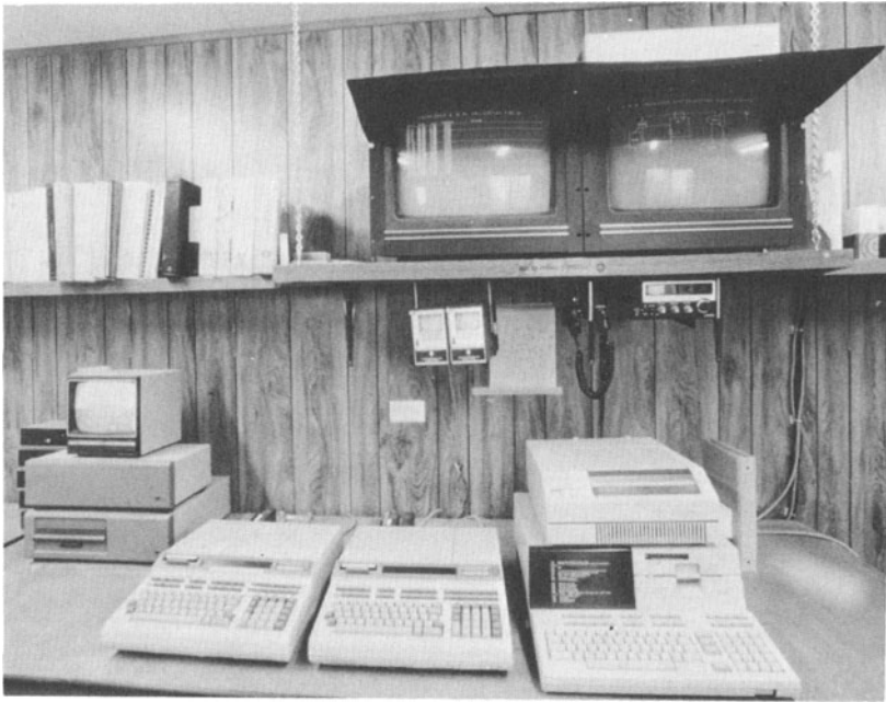
Figure 16. Heliostat Control, Graphics-Data Acquisition, & Steam Generation Control Computers (HP9825, HP9825, HP9826)
