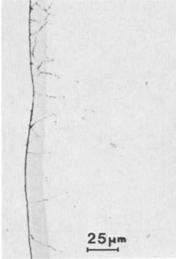
Figure 5 - Nitridation at the surface of a 321 H SS specimen after test in salt containing 1 % BaCl 2 (775 h, 575°C).
